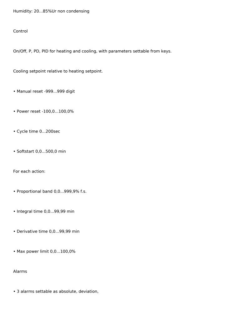
symmetrical deviation to setpoint with direct or reverse function. • Alarm point can be set anywhere on selected scale • Alarms can be masked with exclusion at power-on, with memory, with delayed trip • LBA alarm for setting control • Hysteresis settable for each alarm • Alarm assigned to current input with different operating modes. Weight
